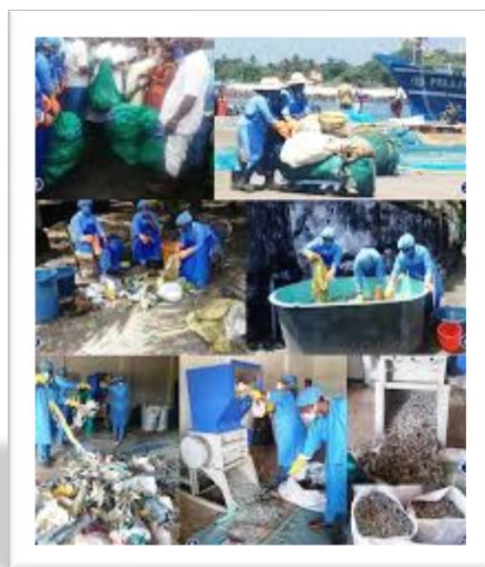
Fig 4.7 Work Flow Collecting Plastic Waste from Sea And Shredding 16
